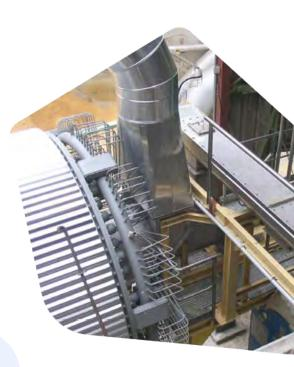
"As the drum also revolves, typical problems of condensation, hot spots, and the hold up of product and bacteria are avoided."
